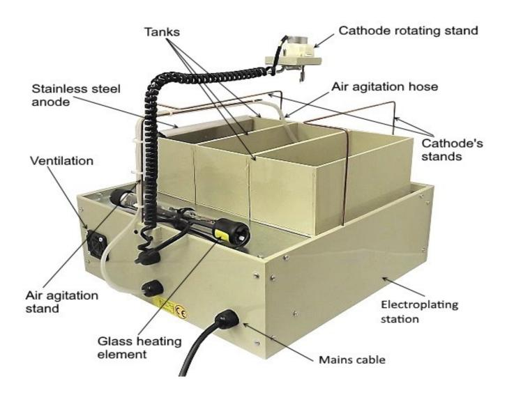
Now you may start any electro cleaning, plating, stripping or forming process by you choose. For this change the Stripping-Plating switch on front panel to "Plating" (for electroplating, electroforming and cleaning processes) position or to a "Stripping" position for a stripping process. This process (stripping) is widely used to remove all residues or unwanted layers from a previously plated object.
