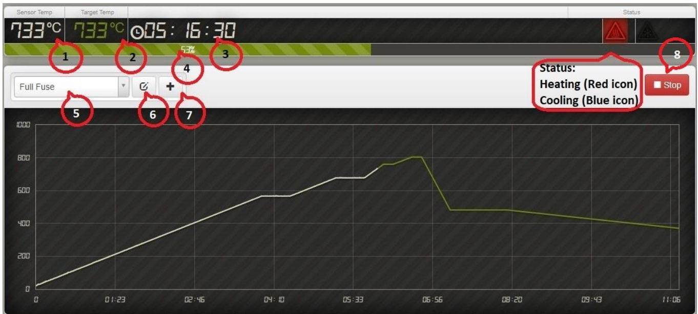
Figure 1. Thermocontroller web interface: (1) Current temperature; (2) Current programmed temperature; (3) Remaining time until program ends; (4) Completion progress; (5) Pre-set program list; (6) Edit selected program; (7) Add/save new pre-set program; (8) Start/Stop button.
